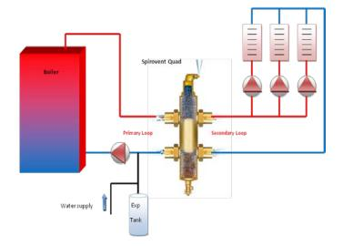
Units must be mounted in straight runs of horizontal piping in a perfectly upright position to allow the vent to operate freely. The piping normally supports the weight of the Spirovent units up to and including 12". Support legs recommended for units 14" and larger. "X" pipe diameters of straight run before and after the unit are not required.
